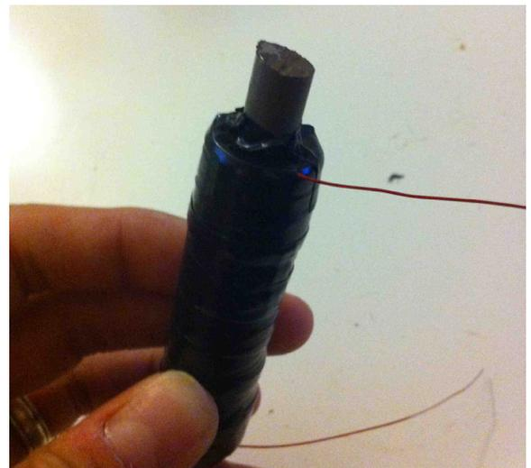
The finished magnet should look something like this. Make sure everything is secure with tape, but be sure to leave the top and bottom ends of the metal rod exposed.
