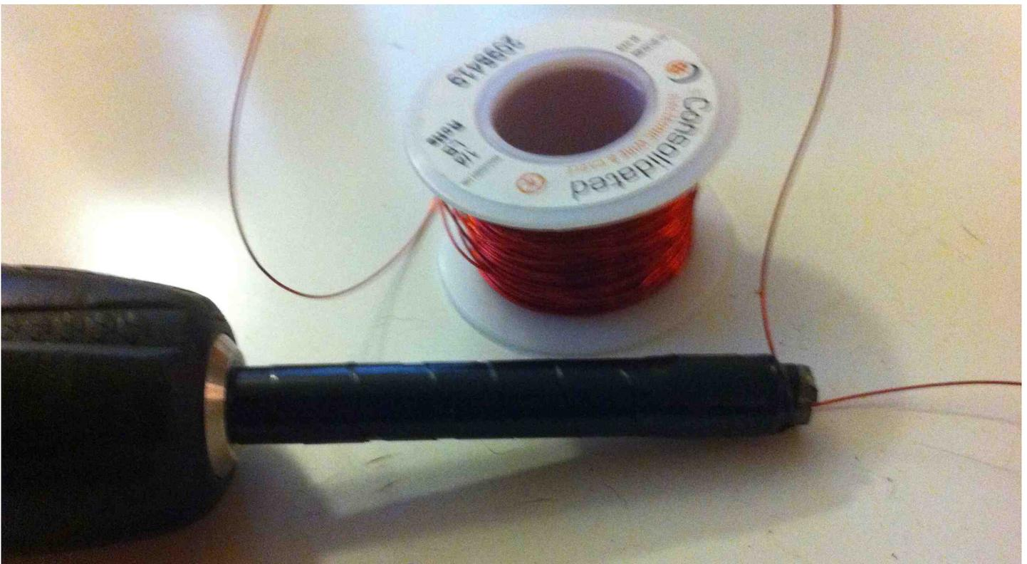
**8.** Repeat this process a few more times. The more wire you wind will result in a more powerful magnet but greater overall resistance. I usually wind my mine until I reach 5 Ohms of resistance. A good rule of thumb is that each up and down wind = 1 Ohm. So going up and down about 5 times is usually sufficient. But anything around 4 – 8 Ohms is good. If none of this makes sense, don't worry and just experiment.
