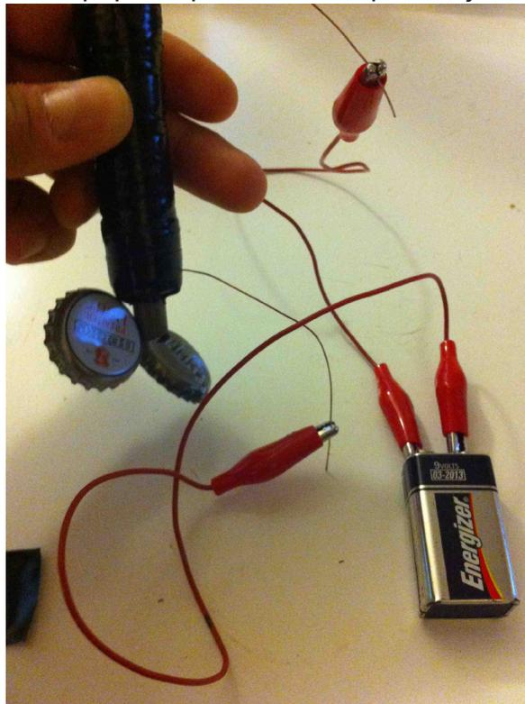
For more power, use more electricity. Try hooking it up to a DC power supply. The increase in available amps will increase the power of the magnet dramatically. But it will also increase the heat it generates. Sometimes it can be hot to the touch so be careful.
