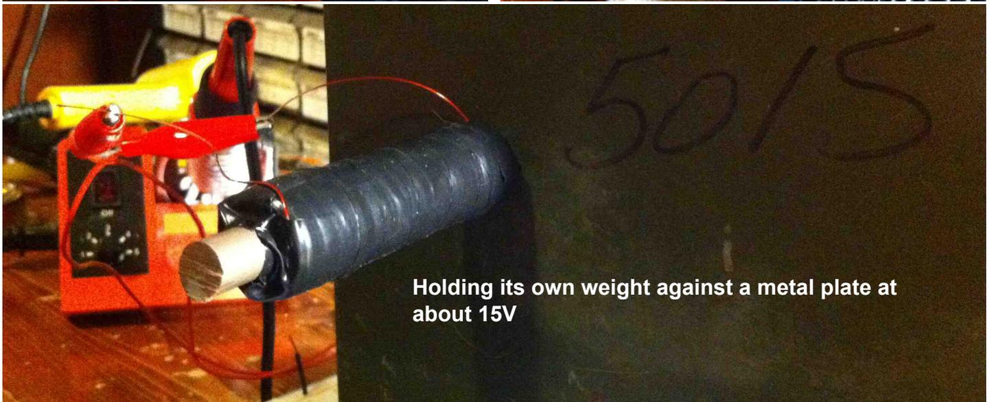
A lantern battery would also work much more efficiently than the 9v. If you're comfortable you can also try a moderately powerful DC wall wart, but don't play around with plugging stuff into the wall unless you are more experienced. **Remember: Batteries can't hurt you, but wall power can!**
