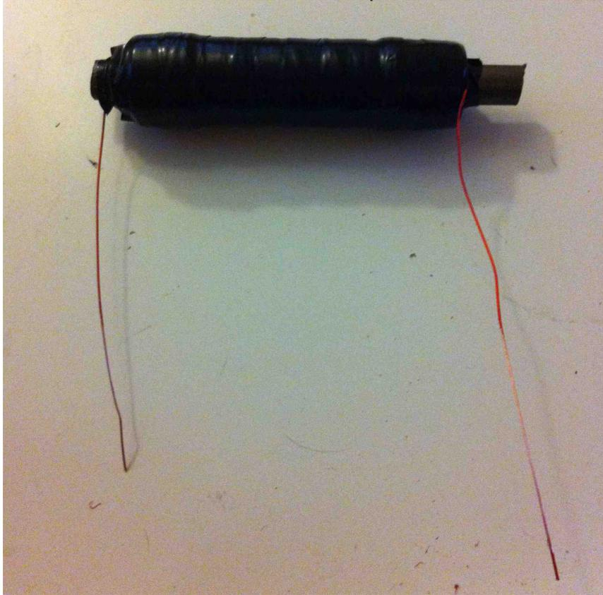
**10.** To test out your magnet, first make sure you have sanded off the insulation on both sides of the wire. Use some clip leads or some wire to attach the + and – of a 9v battery to the two leads of magnet wire. It doesn't matter which side goes to + or – at this point. (Changing that will switch the north and south polarity of the magnet).
