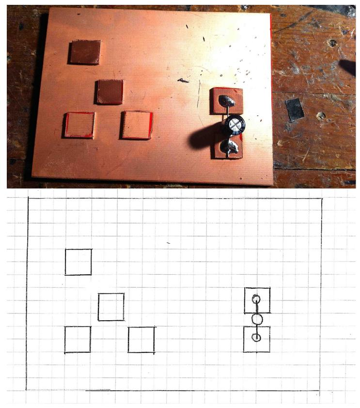
\*\*\*NOTE\*\*\* - This capacitor is polarized meaning that it has to be facing in the appropriate direction. Make sure you solder the NEGATIVE lead to the LOWER of the two squares. The negative side has the shorter lead and a vertical stripe along the side of the capacitor.
