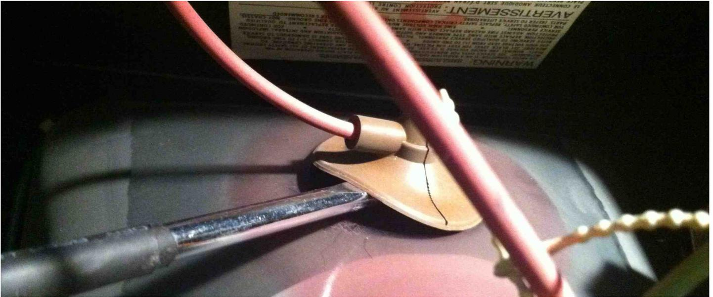
At this point, leave the screwdriver in place for a couple minutes to ensure that all the electricity has been discharged. After that, try discharging it one more time just to be safe. Now you have a safely discharged TV to work with.
