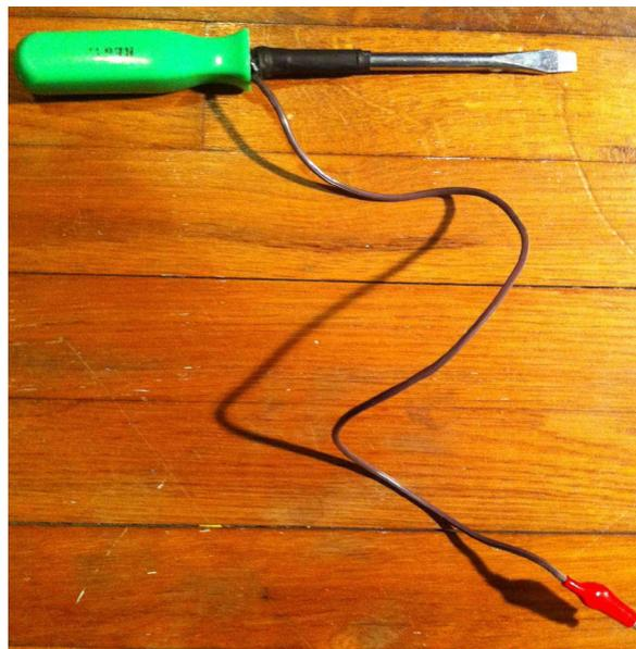
Now attach the other end of the clip lead to the grounding wire or plate of the CRT. This will most likely be an exposed wire that runs around the outside of the tube. It looks like picture hanging wire. If that is not there then it is the metal frame surrounding the tube. The images below show the ground wire and how to attach the clip lead...
